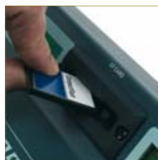
Slot for 32MB Compact Flash cards (play and record functions).
