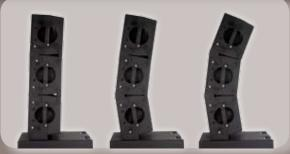
VersArray Series enclosure modules utilize special bracketand-pin flying hardware, a highly flexible, easy-to-rig system that allows full articulation of up to 18 top boxes. With this rigging system, users can adjust two boxes away from each other in 2.5-degree increments from 0 to 15 degrees, providing for a classic line array configuration or a number of angling options.
