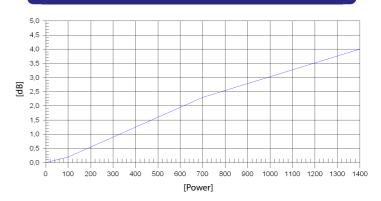
**Note:** Power compression losses were calculated after 5 minutes period applying a pink noise signal filtered between 25 and 200 Hz.
