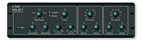
The **3-TAP DELAY** in the X32 records the input signal and then echoes it back after a user-definable period of time and number of repeats. What makes the stereo and triple delay useful and outstanding is the linked tap-timing and musical choice of echo patterns. Use the 3-TAP DELAY to fatten up vocals and instruments, or to add an enhanced spatial element to any performance.
