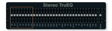
Unlike typical graphic EQs, our STEREO TruEQ delivers the exact frequency response for the new fader setting, taking neighboring fader settings into account – for surgical and responsive filtering or general room equalization (Modeled after BEHRINGER UltraCurve DEQ2496). The XR12 can provide up to 16 mono graphic EQs – one in each of the 6 Aux Buses and Main LR, plus 8 additional mono GEQ effects (4 stereo) that may be inserted into channels.
