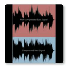
amount of compression for instruments and vocals, creating powerful mixes with punch and clarity. This is indeed a rare feature for products in this class – but standard on the XENYX Q1204USB mixer.
