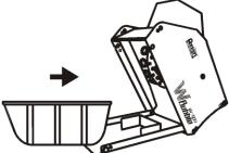
The fluid tank is designed to fit only one way around. Make sure you insert it correctly, as shown above, with the lower edge facing into the machine.
