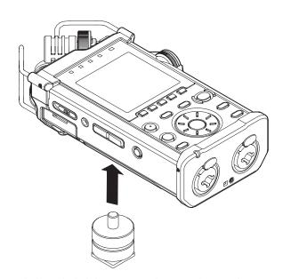
Attach the included shoe mount adapter to the tripod mounting threads on the bottom of the unit to use this unit as an audio recorder with a digital SLR camera or video camera, for example.
