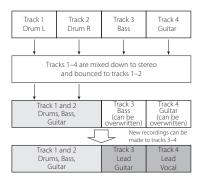
When recorded on the playback track itself, the original playback track is naturally cleared (the drum part in Track 1 - 2 is overwritten in the illustration above).
