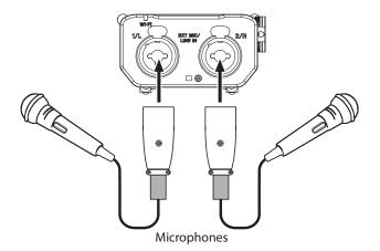
To provide phantom power to a condenser microphone, set the EXT IN switch to MIC+PHANTOM. (See "Set the input gain" on page 19.)
