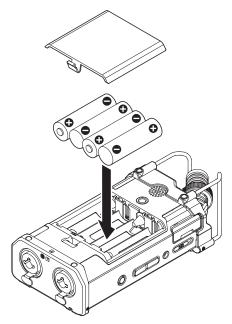
Select the same type of batteries to get an accurate reading of the remaining battery power and required minimum power for operation. (See "Battery type settings" on page 57.)
