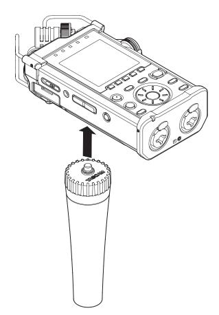
You can attach the included grip to the tripod mounting threads (1/4-inch) on the bottom of the unit and use it as a handgrip. You can also use the grip to attach the unit to a mic stand.
