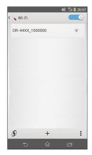
A password input screen appears on the Android device. Enter the password shown on the display of the unit.  Wi-Fi connection is established between the DR-44WL and your smart phone, and the Wi-Fi indicator of the unit will light.
