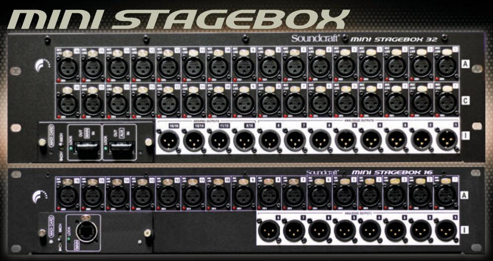
The Mini Stagebox range provides a simple low cost solution to provide I/O expansion for Soundcraft's Si Expression, Si Compact and Si Performer consoles, as well as the larger models including Si1+, Si2+, Si3+, Vi1, Vi2, Vi4 and Vi6.
