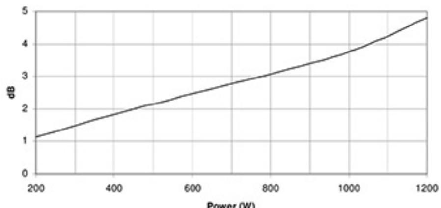
Note: Power Compression Losses were calculated after 5 minutes period applying a pink noise signal filtered between 40 and 200 Hz.
