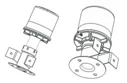
2 Mount solar warning light on traffic cone directly
