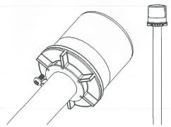
3 Mount on the pier , barrier or the wall
