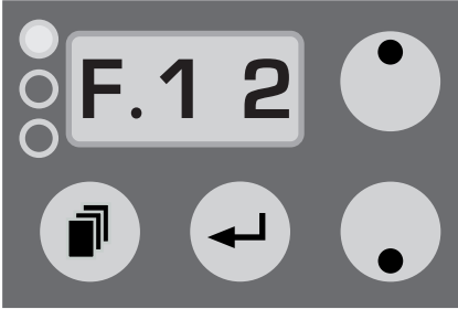
Adjusting of the fog time in seconds (1-99)
