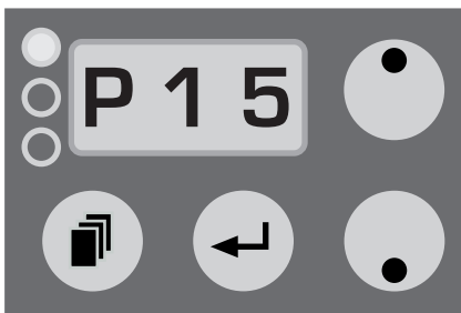
Adjusting of the output/pump in steps of 1% (1-99%)
