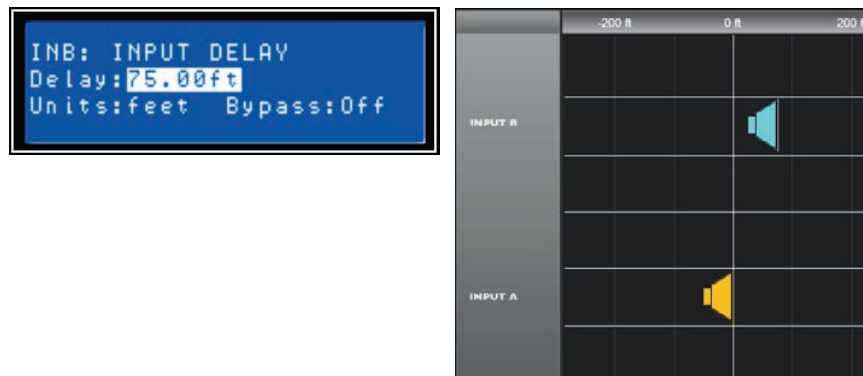
Illustration 5.1: Input B Delay is set to 75 feet. In this illustration, speaker array B is said to be 75 feet in front of Main speaker array A. The effect of air temperature is also automatically calculated for the total delay time using the Temperature value entered in the Setup Menu.
