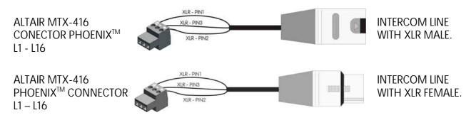
If we used the ALTAIR MTX-416 like audio matrix, we will connect the audio lines L1-L16 to sixteen audio outputs (for normal mode: 4 IN - 16 OUT) or sixteen audio outputs for the inverted mode (REVERSE- 16 IN - 4 OUT). The signal distribution in the PHOENIX<sup>™</sup> connector is the following one:
