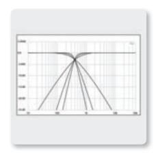
That's why high-quality sound systems use multiple speakers (woofers and tweeters) to spread out the work. While the woofer (usually the larger transducer) does all the heavy lifting, the tweeter can easily handle the high-frequency content. Three and four-way systems distribute the work even more, allowing the individual transducers to reproduce the frequency range for which they were designed. It is the crossover's function to divide these tasks between the various amplifiers and transducers.
