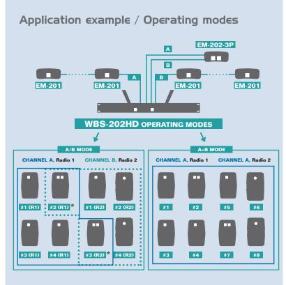
\* Dual channel beltpacks could select communicate with A or B channels individually or with both A+B at the same time.
