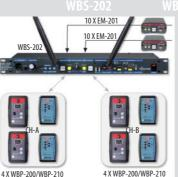
Two groups of 4 single channel beltpacks working in separate communication channels A and B. The base station links and powers another intercom components in both channels.
