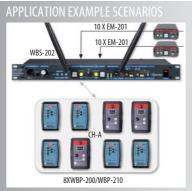
Up to 8 single channel beltpacks in the same communication channel A. The base station links and powers other intercom components in both channels.
